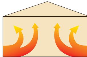
With normal heating systems, the heated air rises upwards outside the usable range.
