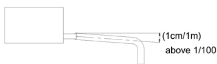
Figure 6.1 Drain piping minimum slope requirement
