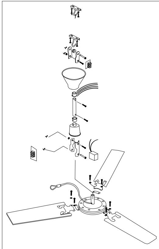
installation, it is recommended that the safety wire is reduced in length to protrude 75mm above the height of the 150mm downrod. The loop for the safety wire will need re-making by using a wire rope grip or crimp (Supplied by others). It is essential that the new safety wire loop will withstand the weight of the fan in the event of it falling.
