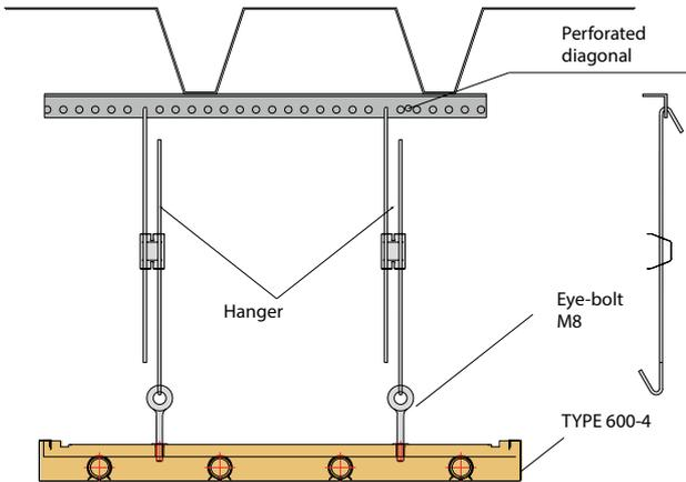
Method D: suspension by using hangers
