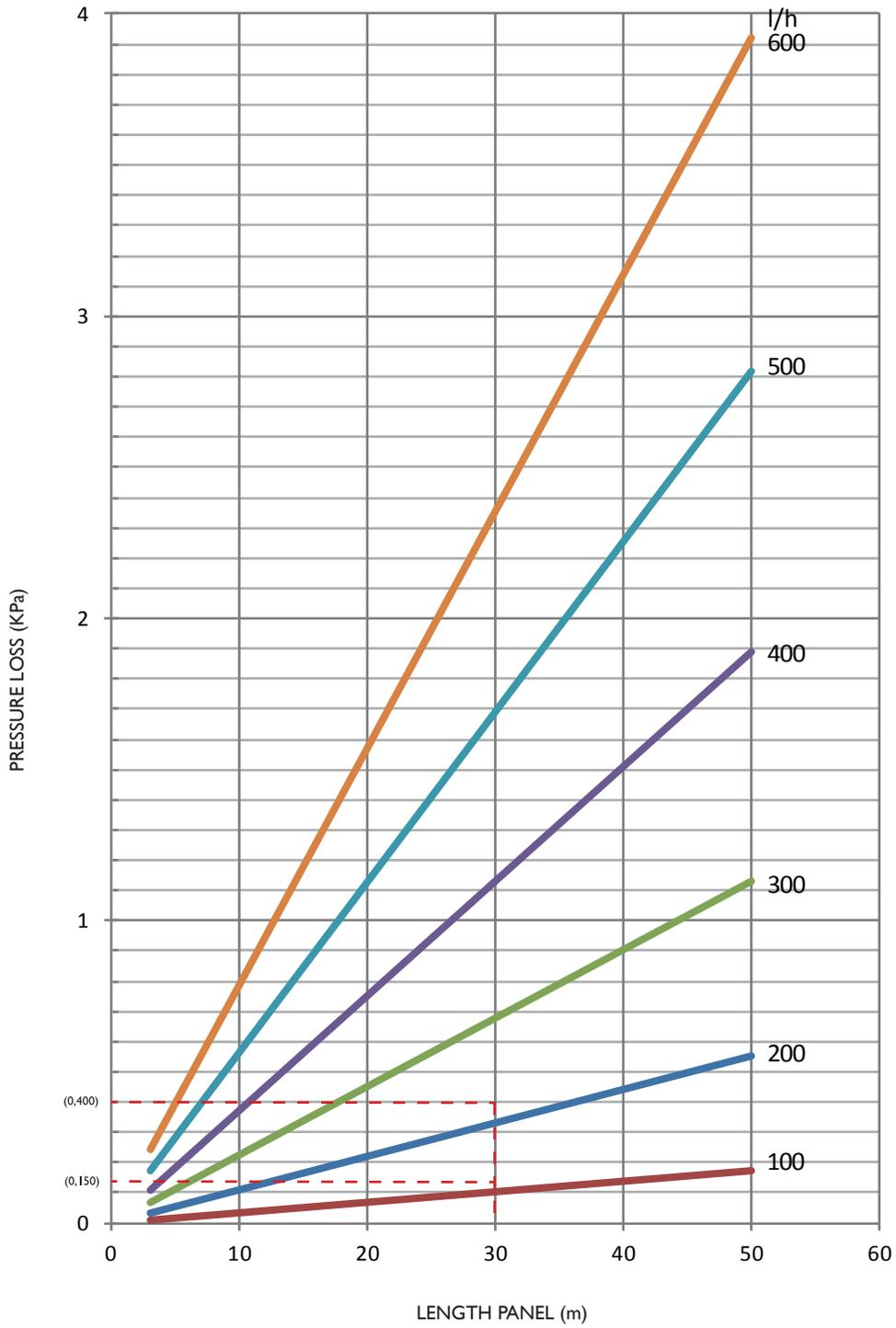
**PRESSURE LOSS IN COLLECTORS AND CONNECTIONS**
