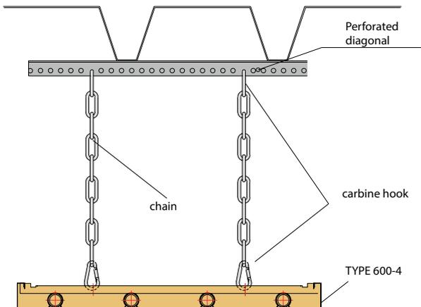
Method F: suspension by using chains an chain tensioners
