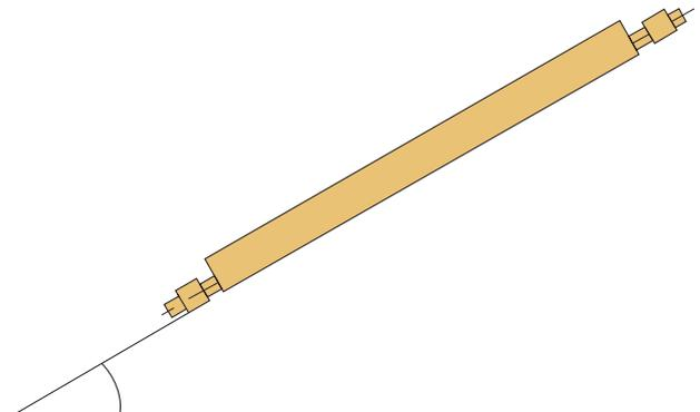
The total output when mounted under an inclined roof is increased by the increasing convection. The correction factor can be determined with the graph on the right.
